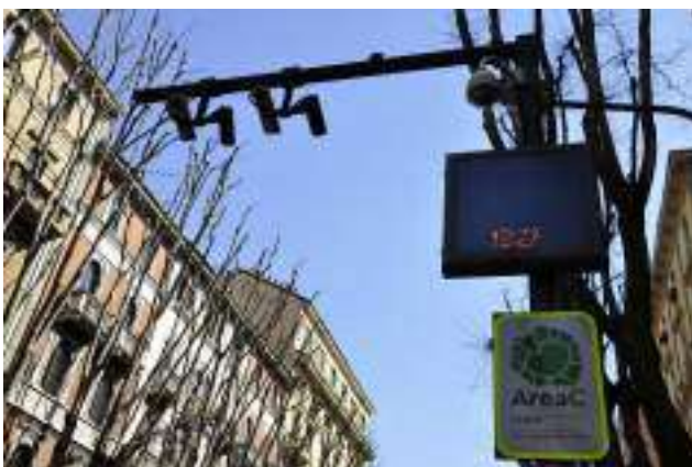
Figure 3 – Camera to control the accesses to Area C
